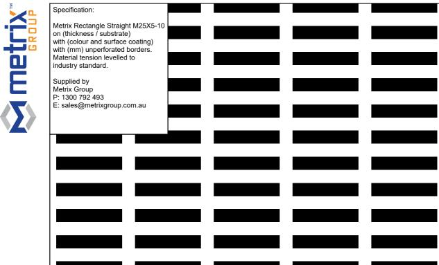
Pattern CodeHole Size% Open AreaRectangle Straight M25X5-1025X5mm42
